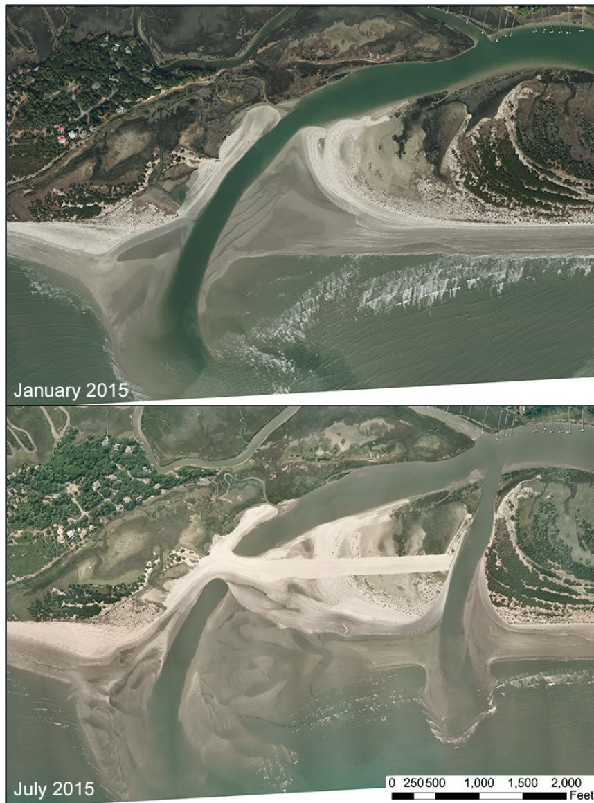
FIGURE 5.1.3a. Captain Sams Inlet before and after inlet relocation in 2015. Kiawah spit is to the right and Captain Sams Creek is at the upper right corner of each image. Ortho-rectified aerial photos were prepared by Independent Mapping Consultants Inc (Charlotte NC).
