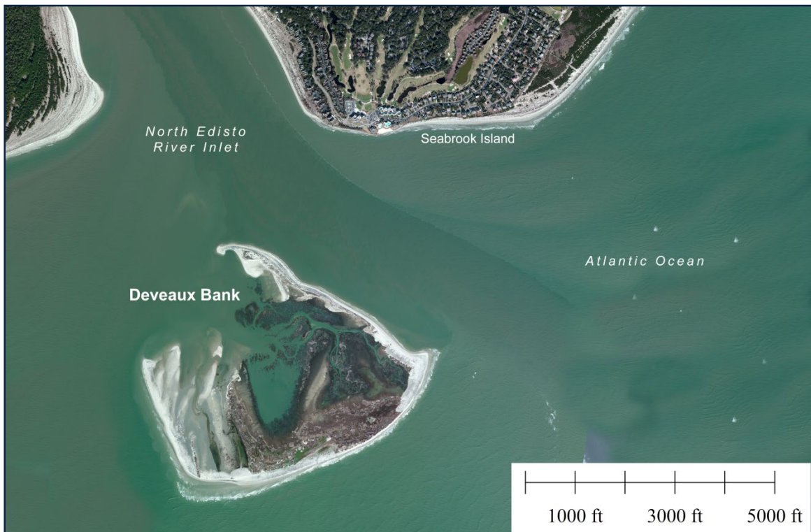
FIGURE 5.2.3b. Aerial photo of Deveaux Bank in 2012. Deveaux Bank is presently a well-established island, which serves as a natural breakwater to the south shoreline of Seabrook Island.
