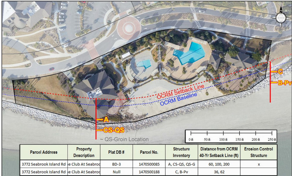
Figure 2.1.3 (f). Two structures at the Beach Club, affiliated with the Seabrook Island Club, are located seaward of the OCRM Setback Line.
