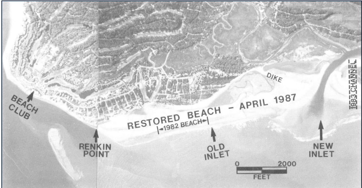
FIGURE 5.1.2e. Seabrook Island in April 1987 after natural restoration by inlet relocation. Area south of Renken Point remained unrestored. (Photo: Courtesy of Seabrook Island POA) [After Kana 1989]
