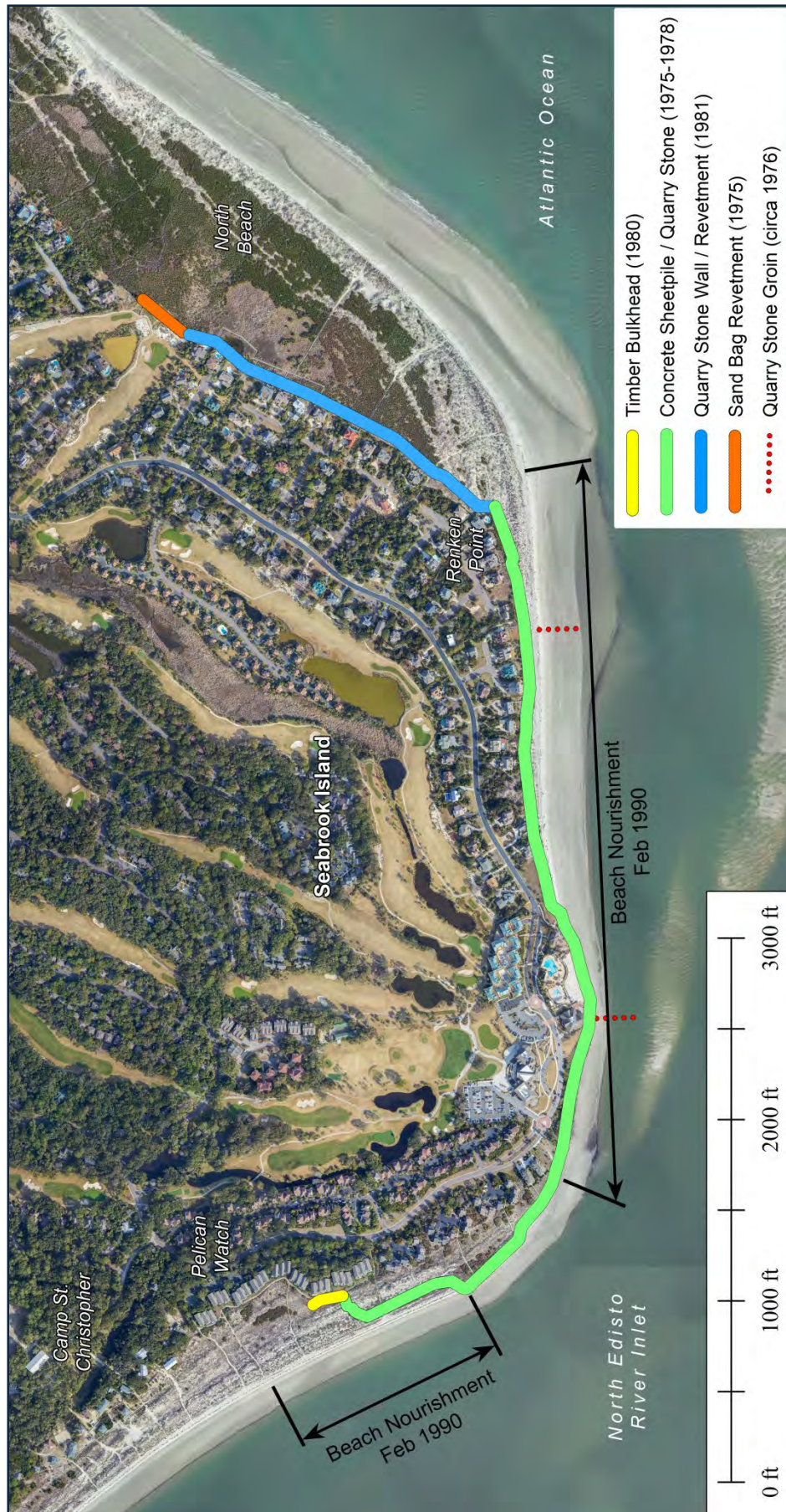
FIGURE 5.2a Location of shore-protection projects along Seabrook Island since the 1970s. Captain Sams Inlet relocation (1983, 1996, 2015) occurred between OCRM 2575 and the Kiawah/Seabrook Town easement line (outside image range, see Fig T-3).
