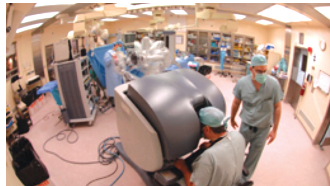
Figure 2 (RIGHT) From: https://clinicalcenter.nih.gov/dpms/imri.html . Shows in the foreground a console where the surgeon performs a robotic laparoscopic operation. Anesthetized patient is in the background with robot. Department of Perioperative Medicine of the NIH Clinical Center.
